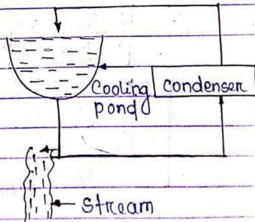
→ The water from the condenser is stored in the earth like ponds where natural evaporation brings down the temperature.
