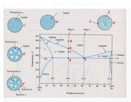
Match the expected phases present at points a,b,c,e,f with the schematic microstructures shown against b',c',d',e',f'
