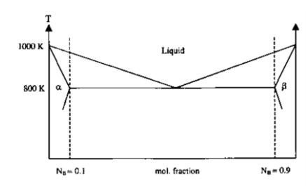
In the above hypothetical phase diagram, the melting point of each pure component is 1000 K and the cutectic temperature is 800 K. The cutectic is located at the equi-atomic composition. The maximum solid solubility in  $\alpha$  phase is given by mole fraction  $N_B = 0.1$ .
