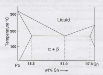
A Pb-Sn hypo-eutectic alloy is slowly cooled from the liquid state to room temperature. The composition of the alloy whose microstructure consists of 25 wt% lamellar constituent is
