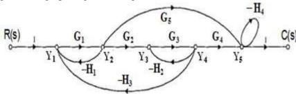
24. Represent the block diagram of Figure by its SFG.
